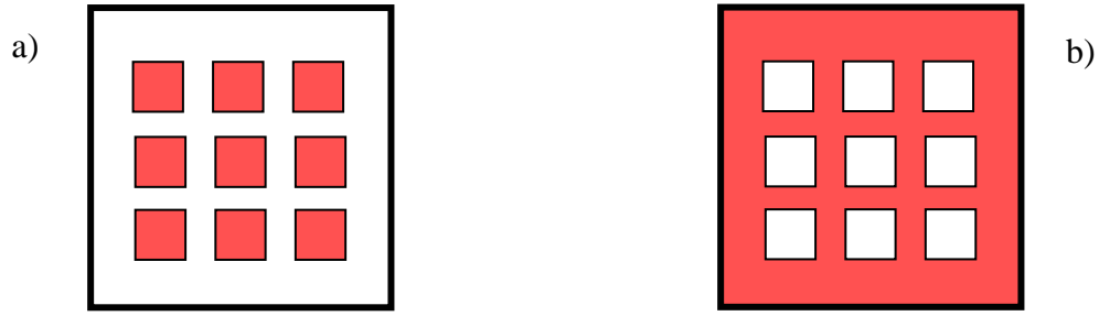
Fig. 5.2. A mask layout can be converted to hold the mask itself or its background. A set of squares in the layout can result in a set of squared “mesas” in photoresist or a set of squared holes in a photoresist layer.
