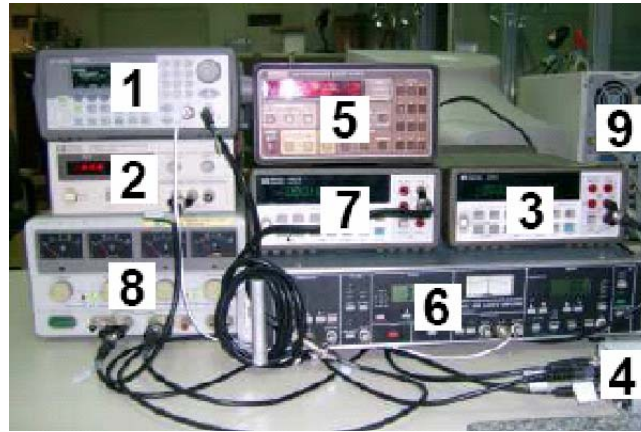
Fig. E1. Instrumentation required for magnetic label detection. Magnetic field excitation: 1, function generator (HP 3220A); 2, dc power source (HP E3612A DC); 3, amperometer (HP 34401A); and 4, Current control box (custom-made). Sensor power supply and readout: 5, dc power source (Keithley 220); 6, lock-in amplifier (EG&G Princeton Applied Research 5209); and 7, voltmeter (HP 34401A). Multiplexing power supply: 8, dc voltage supply (GW GPC-3020 DC). Control and data acquisition: 9, PC with Agilent GPIB card and NI DAQ PCI6024E. An additional function generator (PM 5132) is also used as a power supply for current lines. Also, BNC and GPIB cables are required for connections between instruments and control boards.
